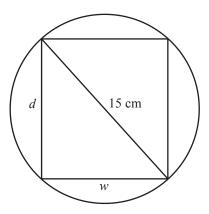
The strength *S* of the beam is proportional to the product of its width and the square of its depth.
